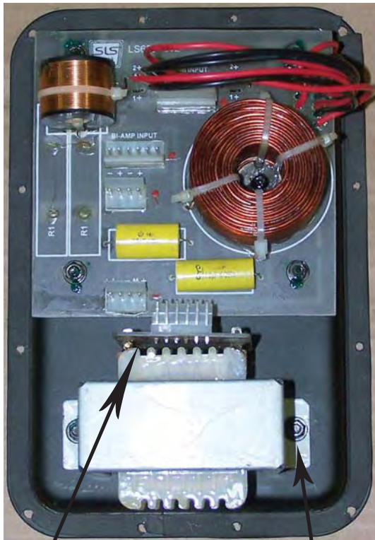
Transformer Circuit Board facing Crossover
